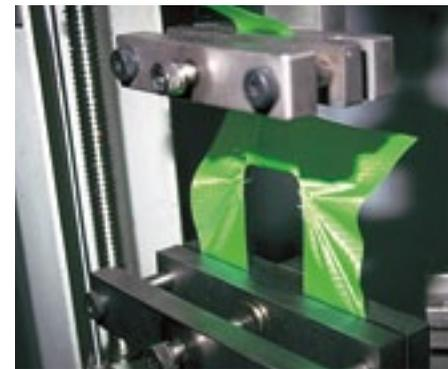
Testing the resistance of the Kerlon fabric.
